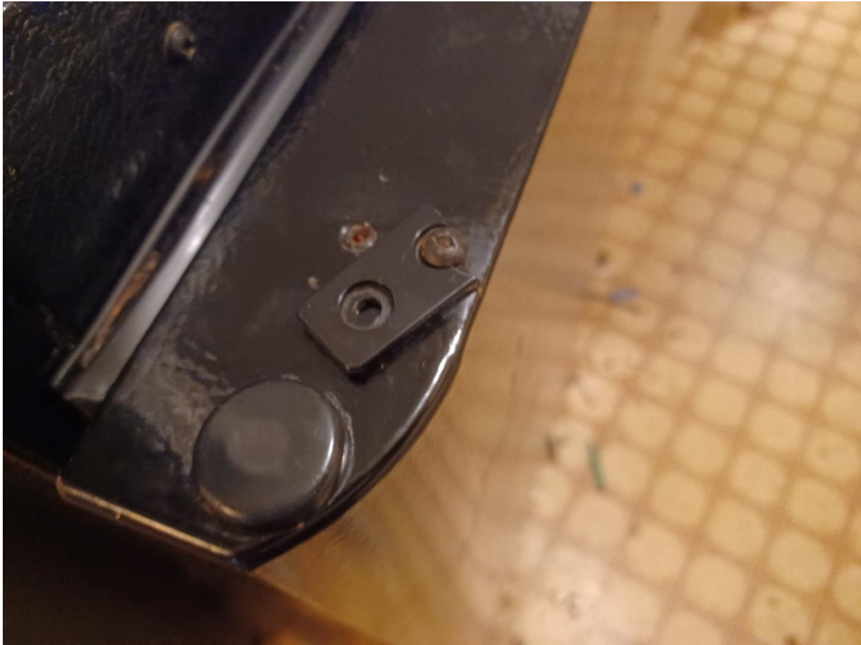
Refrigerator door handle broken off. Arrows show where mounting holes are located.
